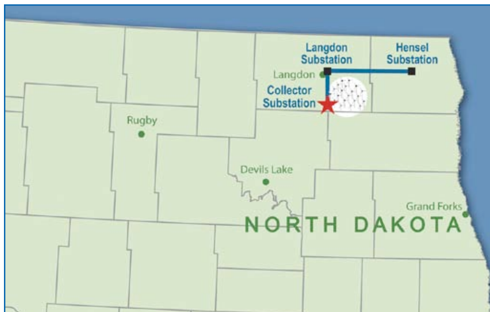
The existing 35 miles of 41.6-kv line between the Langdon and Hensel substations will be upgraded to 115 kv to help transmit the electricity produced at the Langdon Wind Energy Center.
